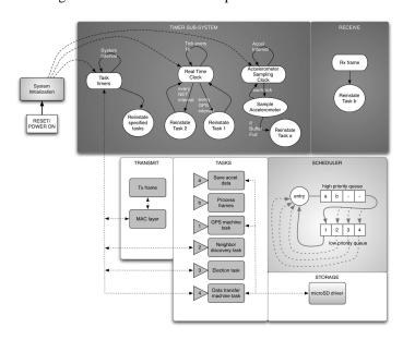
Fig. 4. Top level block-diagram of the CARNIVORE firmware.
