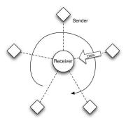
Fig. 6. Round robin star network. The receiver mediates the round-robin data transfer, accepting data from the senders. Either sender or receiver can end the transfer.
