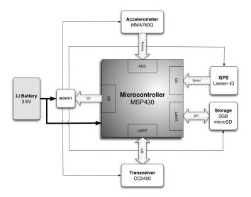
Fig. 2. Top level block-diagram of the CARNIVORE hardware. Black arrows indicate power connections. Thick, shaded arrows indicate control and data connections.
