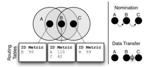
Fig. 7. Hidden-station example. Radio range is shown by the shaded circles. A nominates B, B nominates C, and C nominates itself in the election. B ignores A's nomination and A times-out. C accepts B's nomination. B then sends data to C and A does not transmit any data during this network wake-up.
