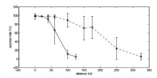
Fig. 8. Range test results for CSN-to-CSN (solid line) and CSN-to-SRN (dashed line). Bars indicate one standard deviation.
