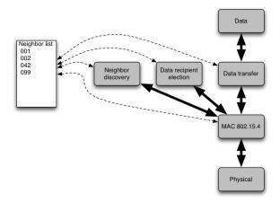
Fig. 5. Network stack and associated data structure. The CARNI-VORE stack uses a routing table of neighbors. The list is populated during neighbor discovery and updated by various layers. Received frames are processed in the MAC layer which then updates the neighbor list.
