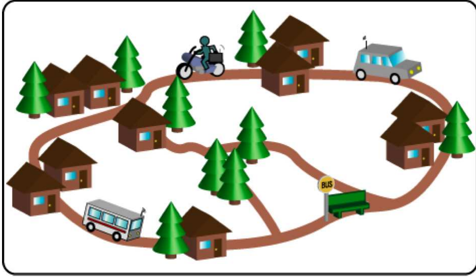
Figure 2.1: A sample village scenario with various types of mobility. The mobility of vehicles tend to exhibit patterns such as recurring paths. The path information can be leveraged to make more informed routing decisions in a hop-by-hop opportunistic manner.
