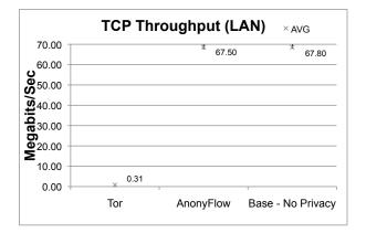
Fig. 4. TCP Throughput (iperf) between the 2 hosts in our testbed.
